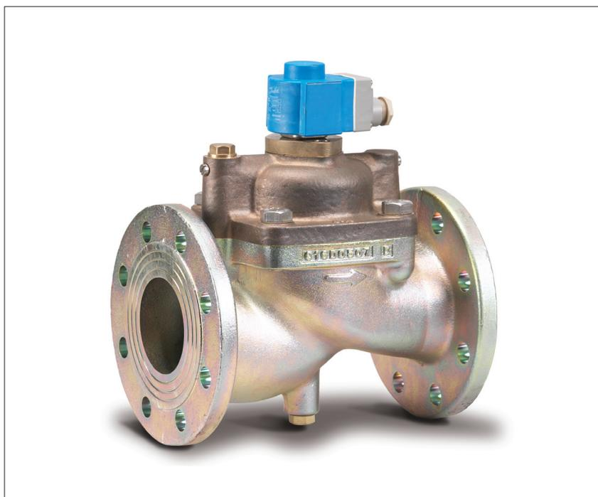
EV220B 65 - EV220B 100 is a 2/2-way solenoid valve program for use in robust industrial applications, demanding high flow rates. The valve is designed with cast iron valve body and flanged connection. Water-hammer damped design and built-in pilot filter ensures a reliable operation.
